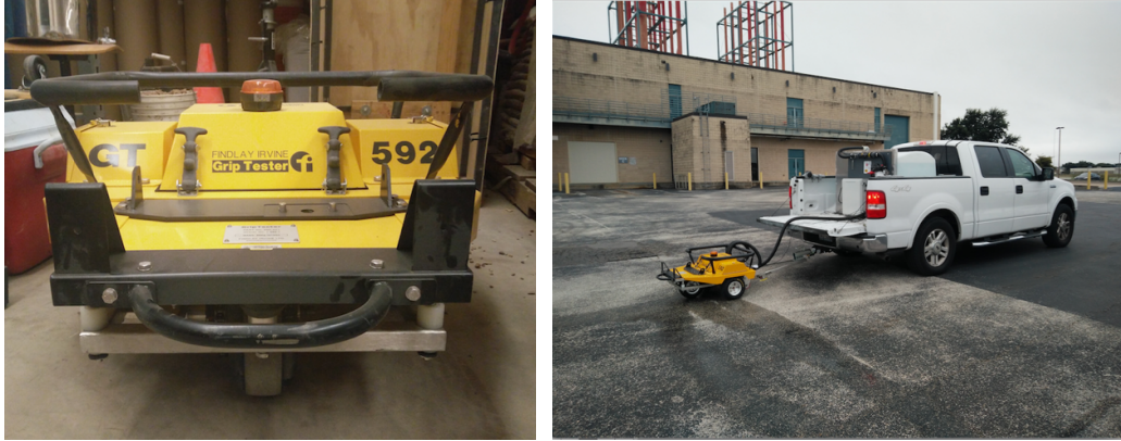
Figure 2.16: (a) GripTester, and (b) field operation.
