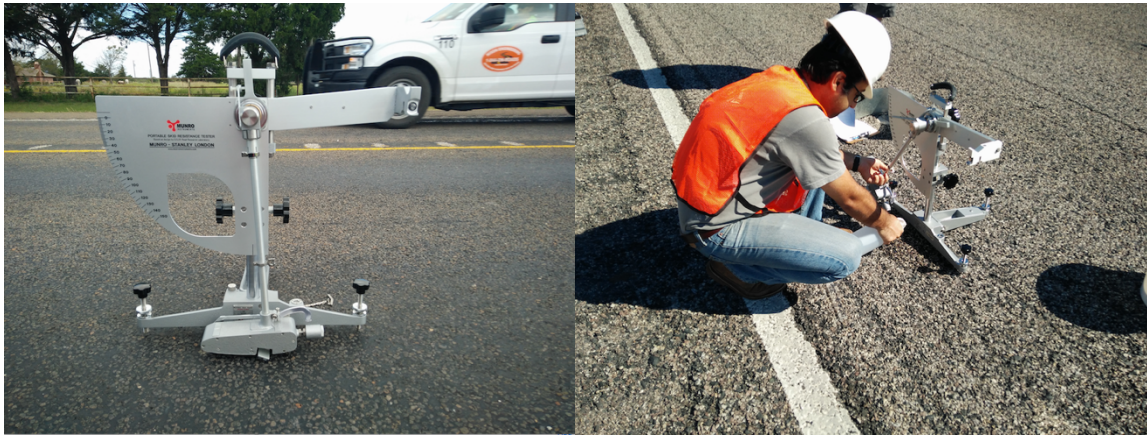
Figure 2.14: (a) British Pendulum Tester (BPT), and (b) field operation.
