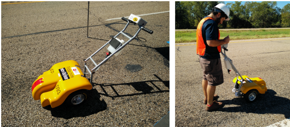
Figure 2.17: (a) Micro GripTester, and (b) field operation.
