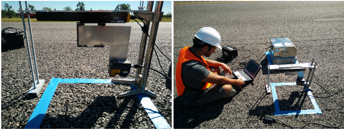
Figure 3.3: (a) Line Laser Scanner (LLS), and (b) field data collection.
