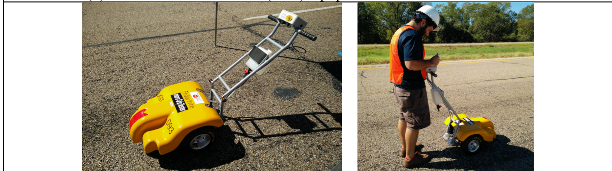
(c) Micro-GripTester equipment and field data collection
