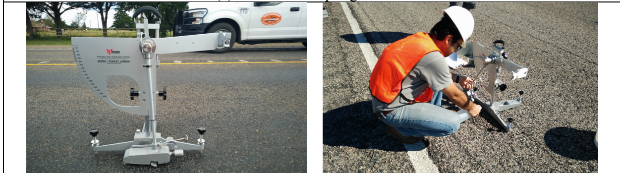
(b) British Pendulum Tester (BPT) equipment and field data collection
